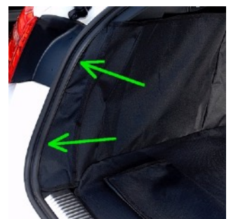
Figure 3 - Tuck leading edge behind rubber seal
