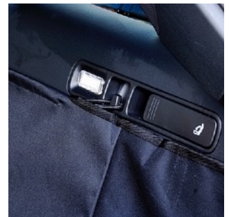
Figure 1 - Plastic hook attaches to seat locking point
