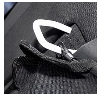
Figure 1 - Plastic hook attaches to seat locking point
