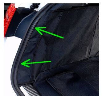
Figure 3 - Tuck leading edge behind rubber seal
