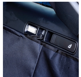
Figure 2 - Bungee eye attaches to side hook
