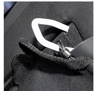
Figure 1 - Plastic hook attaches to seat locking point
